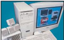
Based on the 800MHz Athlon, this PC has an Asus A7V motherboard, a 1GHz processor and has a 200MHz FSB augmented by 128MB of PC133 SDRAM. There is a 15.3GB IBM hard drive, as well as a Teac CD-RW drive and an eight-speed DVD-ROM drive for movie playback. It's also great for video-in-and-out functionality with a Prolink TV-tuner card.
