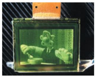
Television from Seiko-Epson using a 2in organic screen from CDT with a resolution of 800 x 236 pixels
