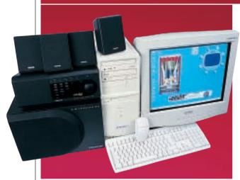
LIKE THE PANRIX, Atlas and Mesh, Polar's entrant features a 1.1GHz Athlon processor. This finds a home on an Asus A7V motherboard, complete with 256MB of PC100 memory. This time, though, the memory has been divided into two modules. This leaves one memory slot for future upgrades. With this arrangement the overall SYSmark score is a fairly average 187.
