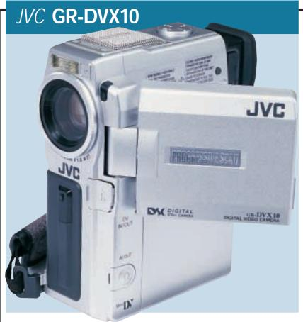
THE SMALLEST OF THE camcorders in this group test, JVC's GR-DVX10, is a compact palmcorder that, despite its diminutive appearance, is packed with features. Many of them come courtesy of the DVX-10's 8MB multimedia card that allows you to take digital still pictures while simultaneously shooting video, recording and audio dubbing MP3 sound effects and creating compressed, short video clips for emailing.
