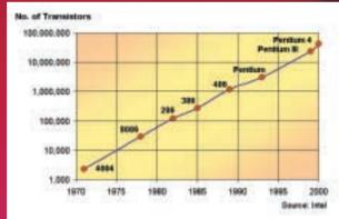
Pentium III processor contained over 27 million transistors. Early versions of the Pentium III, and for that matter AMD's Athlon processor, were manufactured using a 0.25micron process. The latest models from both companies now employ a finer 0.18micron process and this is set to reduce even further over the next year. It may not be too long, though, before CPU growth starts to slow down
