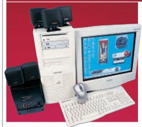
THE MOST INTERESTING aspect of the 1100W is the inclusion of an UltraDMA100 EIDE-RAID controller from Promise. There are a number of RAID types and Panrix has opted for striping (Level 0). Using this method increases disk throughput as the two 40.9GB Maxtor drives have independent roles - one is used for read and the other for write operations. This halves the access time resulting in a system that runs at an impressive speed. In addition, the
