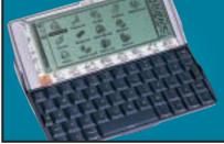
The Psion 5mx is a quality PDA weighing 354g. It has a screen resolution of 640 x 240, a serial connector for syncing with your PC and space for upgrading with Flash memory. The keyboard is excellent and responsive, ideal for its word processing capabilities. With 16MB of memory and 15MB of Flash memory this is an ideal handheld computer.
