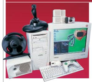
TIME HAS CERTAINLY fulfilled our criteria by supplying a machine built around a beefy 1.2GHz Athlon processor backed up by 256MB of PC133 memory. The latter comes as two 128MB modules, which leaves one slot free for memory upgrades.
