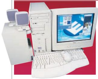
**DELL IS ONE OF** three manufacturers this month to opt for an Intel-based solution. A 1GHz Pentium III processor sits in the socket of a Dell-badged 815E motherboard and is backed up by a healthy 256MB of PC133 memory. A well-designed internal cooling system helps keep the temperature down inside the case but we did find the cabling rather untidy.
