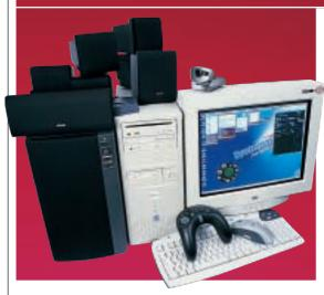
THIS IS THE SECOND machine in this test to use the already outranked 1GHz Pentium III housed in an Intel 815Ebased motherboard - the CUSI 2 from Asus. With 256MB of PC133 memory occupying one of the three DIMM slots, you'd expect the P1000RV to be a fair performer, but like the Dell it finds itself hanging about the lower half of the SYSmark graph, with a score of 181.
