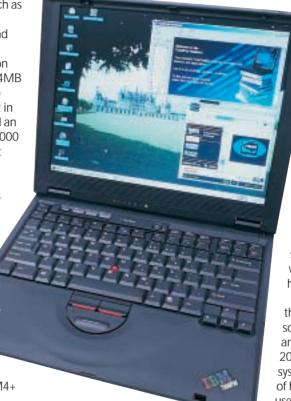
keyboard. This can take a little time to master fully but it does afford a precise way of moving the arrow around the screen. Beneath this, in addition to the standard selector buttons, is an additional button that, when pressed, allows you to scroll through pages with the trackpoint.
