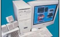
Built on the Asus A7V motherboard this PC has a 900MHz Athlon, 128MB of PC133 memory, a 40GB Maxtor DiamondMax Plus hard disk and a BURN-Proof CD-RW. Its DVD is a slot loading AOpen drive, while graphics are covered by a 32MB Radeon. With video piping out to the Mitsubishi Diamond Plus 91 19in monitor this is an excellent mid-range system with Windows Me.
