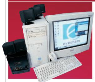
THIS HAS ALL THE makings of a very fast machine. Under the lid is a 1.2GHz Athlon plugged into an Asus A7M266 motherboard. This board really unleashes the power of this Athlon as the AMD 761 North Bridge supports a 266MHz front-side bus (FSB), to match the processor. Together with the single 256MB stick of PC2100 DDR SDRAM this lifts the SYSmark score to 210 - the top spot.
