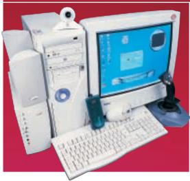
**NEC'S DIRECTION** is the same price as the Mesh, and in terms of value for money there's little to separate them. Both have 256MB of PC133 memory. and where Mesh has offered a faster Athlon processor and a quality sound system, the Direction fights back with two 46.1GB hard drives, a range of peripherals (joystick, webcam, TVtuner) and some extra software.
