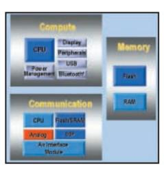
sized memory modules shown by several vendors at Comdex we're reviewing one next month. MSA would essentially replace all but the Air Interface section of the Comms module, providing a relatively simple programming interface. The air interface consists of chipsets for GSM or other wireless technologies
