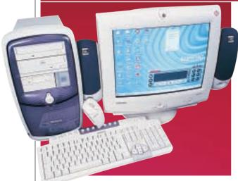
THE PRESARIO'S CASE has an interesting style, with a front panel that drops open to reveal space to store several CDs. On the inside, the core is a 1GHz Athlon processor, coupled with 128MB of PC100 memory. Compared to the others on test this is a bit stingy and we would have preferred to have seen 256MB of PC133 memory instead, since the VIA KT133 chipset on the motherboard would be able to take full advantage of it. Storage is taken care of
