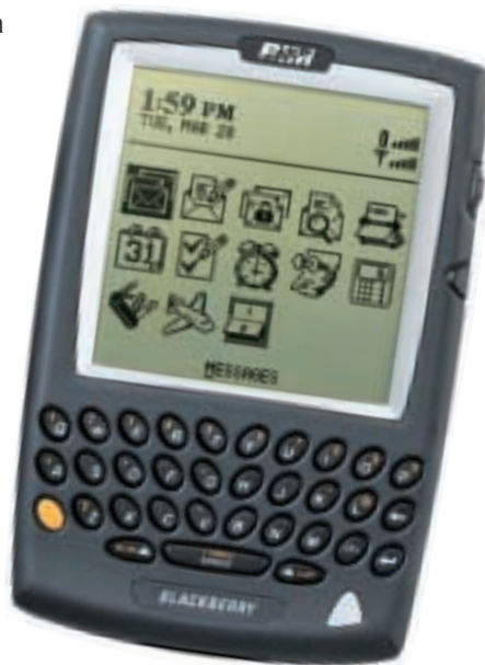
The Blackberry from RIM is aimed at the business market – it's already a success in the US on a two-way paging network. Intel-based, it holds the promise of a gaming future
