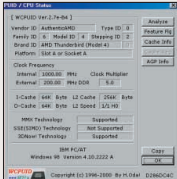
H Oda's legendary WCPUID utility is an invaluable tool for identifying types of CPUs – in the screenshot, note the 1,000MHz Athlon has a Thunderbird core
