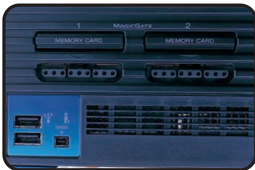
You'll find a host of ports on the PS2 – two USB ports and a FireWire port – which will open up opportunities for all manner of peripheral connections
