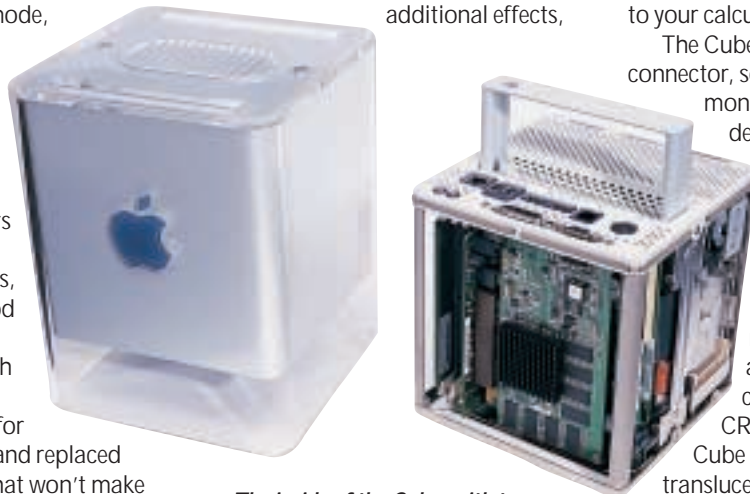
The inside of the Cube, with two spare memory slots
