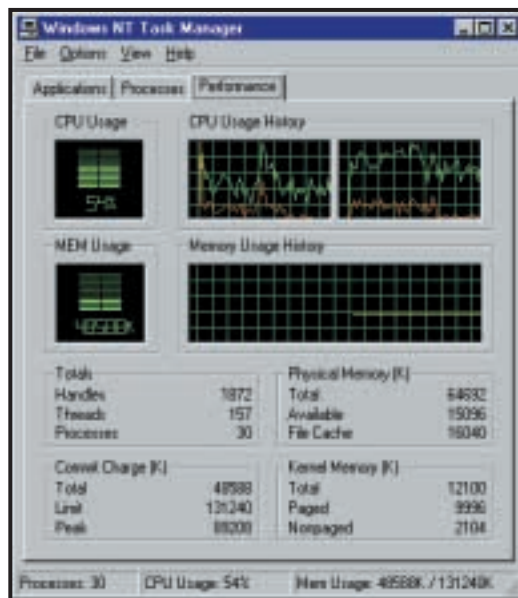
Instead of displaying one graph that tracks CPU utilisation, in a dual CPU PC you get a pair. Here, Windows Update is revealed as a CPU-hungry task
