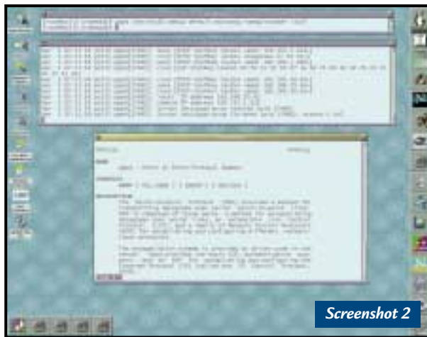
Run your pppd experiments under X (but as root, of course) and you can run tail -f in its own xterm, while starting and stopping pppd in another window
