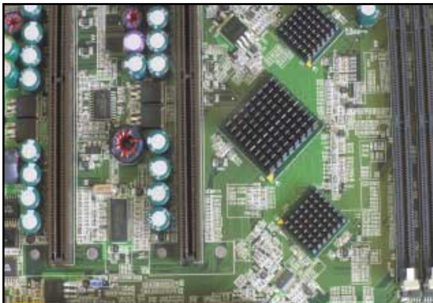
Intel's top of the range 840 chipset, pictured here on a Supermicro PIIIDME motherboard. Note the 45 degree orientation of the chipset components to ensure track lengths are exactly correct, and MTH support for SDRAM DIMM slots on the right. Even with dual memory channels though, is the 840 the best chipset for SDRAM performance?
