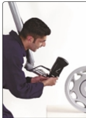
Broadband links may boost the use of 3D on websites, with it the demand for this ModelMaker scanner, which pumps 3D models of real-life objects into CAD packages. It's one of a range from Coventry-based 3D Scanners and costs up to £1m.
