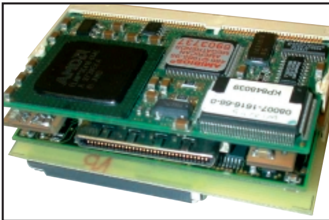
A tiny PC from the Stanford site and yes, that is one of the IBM microdrives just visible on the bottom of the device
