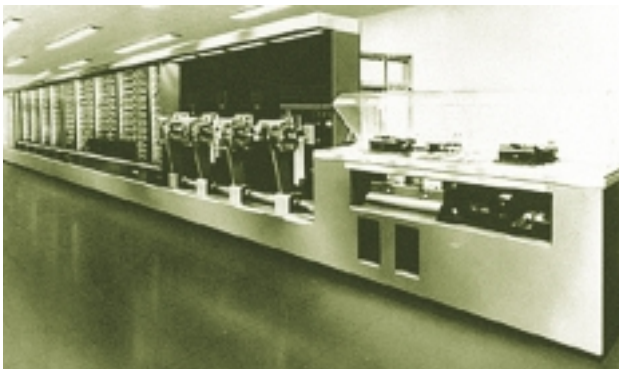
Frame up... IBM's five-ton 1944 Automatic Sequence Controlled Calculator, or Mark I, developed in co-operation with Harvard University, helped give the company an early lead in the mainframed post-war world
