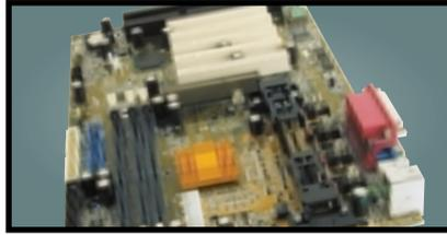
This board has four PCI slots, one ISA and one shared slot. It was very stable in our tests and the manual spells out clearly what the jumpers do and takes you through each of the Award Modular BIOS settings step by step.
