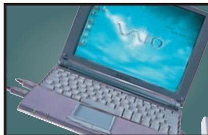
The 505X has a very thin casing but still packs in a Celeron 333MHz processor, 64MB of RAM and a 6.4GB hard disk. A screen resolution of 1,024 x 768 offers crystal-sharp images and text. Peripherals can be connected via the built-in USB and FireWire ports or Type II PC Card slot. The 505X is a great evolution of the ultra-portable notebook format.
