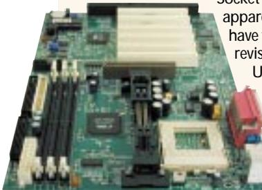
jumpers to set the multiplier, which is fiddly and could have been done with switch blocks or software-controlled options. The manual did not specify the configuration for a multiplier of 7.5, which the 500MHz Celeron requires, so we set it to 7. Since the Celeron is multiplier-locked this wasn't an issue. Another problem was that pin one on the front panel connector had been incorrectly labelled.
