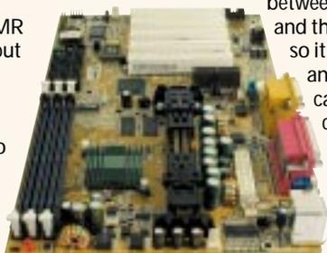
connectors are two PS/2, two USB, one serial, one parallel, one D-SUB video, one game port and audio in, out and mic. A riser is provided for the second com port so if you need to use this you don't need an extra cable.
