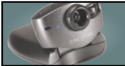
Not only is this a regular webcam offering 30fps at 352 x 288 or 15fps at 640 x 480, but when you disconnect the USB cable it becomes a standalone digital camera that can store JPEG images on its internal 4MB memory.
