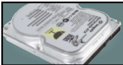
This 28GB beast's spin speed of 7,200rpm helped it achieve 0.89Mbytes/sec in our random read and write test. It's a breeze to install and the £5.10 cost per MB makes it a bargain.
