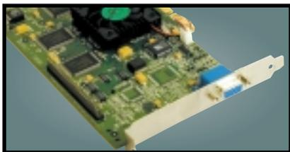
Based on the DDR version of the GeForce 256 chipset from nVidia, this card offloads transform and lighting effects processing from your CPU to give outstanding results.
