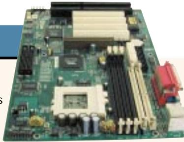
**Socket 7** This Super Socket 7 motherboard is based on the VIA MVP3 chipset, which can support up to 2MB of on-board cache. This board comes with either 1MB or 512KB, so check before you buy. It has the advantage of accepting both SIMMs and DIMMs – there are two SIMM and three DIMM slots.
