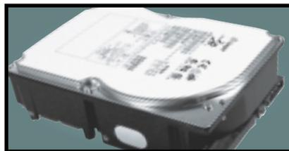
The Barracuda may no longer be at the cutting edge of SCSI performance, but with its 7,200rpm spin speed and 50GB storage space its value for money is outstanding.
