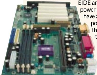
of the major components and allow for a user-friendly upgrade path. There are four PCI slots and one shared slot, plus the standard single AGP slot. There's also an AMR slot that is unusually positioned below the AGP slot.
