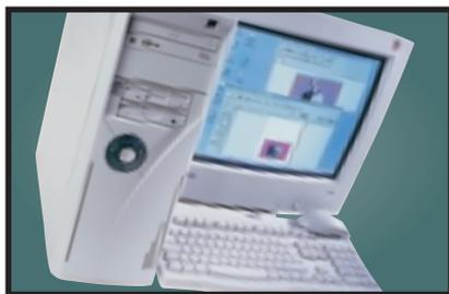
Built on an 820 chipset, this speedy machine uses the 0.18micron 733MHz Pentium III. It comes with a single 256MB DIMM for memory and a Guillemot 3D Prophet graphics card with 32MB on-board. For storage, a Zip 250 drive and a 27GB Maxtor UDMA66 hard drive are included alongside the Pioneer DVD-ROM. You also get a large 19in monitor for your money.
