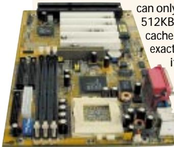
This model is laid out well, with EIDE, floppy and ATX connectors in
