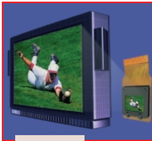
▲ SMALL IS LARGE: MICRO DISPLAYS CREATE A TINY IMAGE WHICH CAN BE BLOWN UP TO NORMAL SIZE
