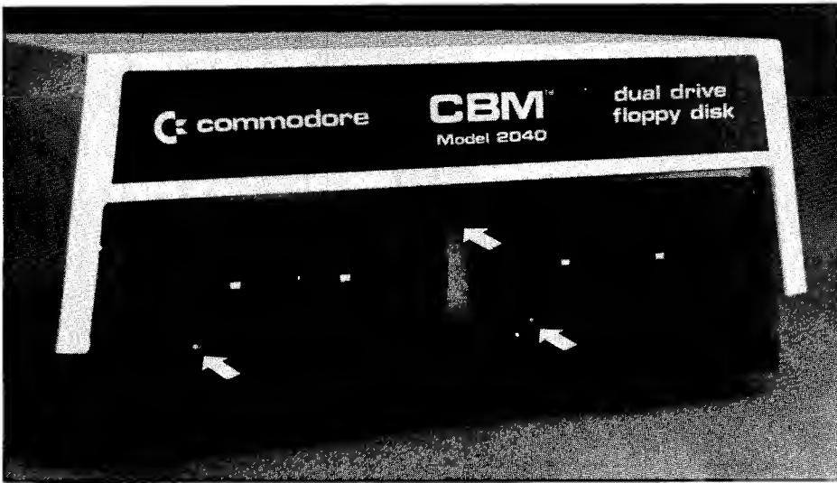
Figure 1-22. Dual Drive Floppy Disk LED Indicator Lights
