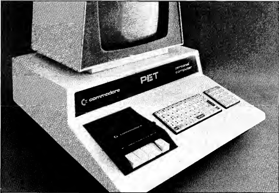
Figure 1-10. PET 2001 Internal Tape Drive
