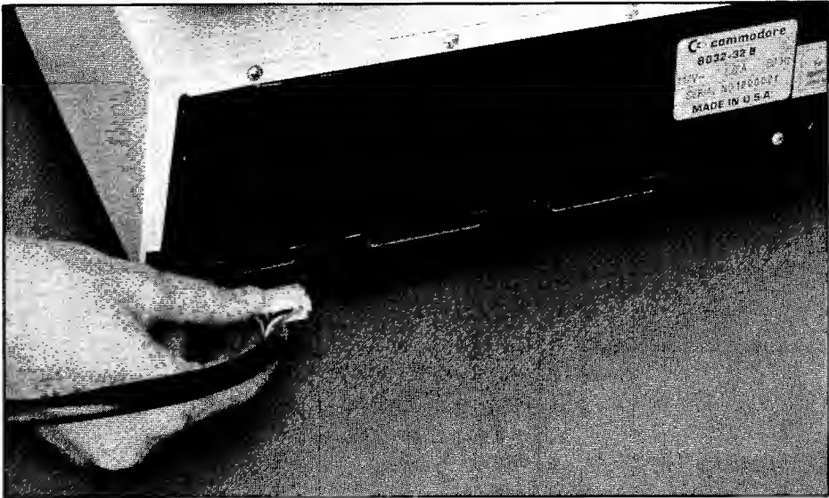
Figure 1-12. Connecting Second External Cassette Unit to CBM Computer
