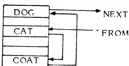
The head of the list which points to the first data item in the chain is held in the first location in the table. The last item in the chain points back to the head of the chain. The program puts each data item in the next free place in the table and links it into its place in the chain.
