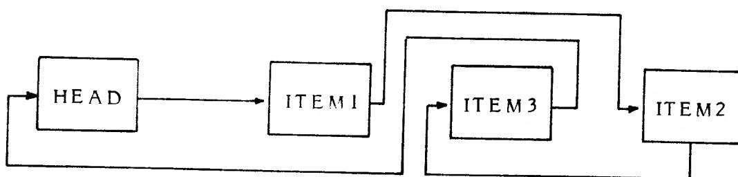
If data is held in a table like this, a user can output the data either in the sequence in which it is held or in its chained sequence. Each item input is compared with items in the chain, starting from the head of the chain, and is linked into its correct position.
