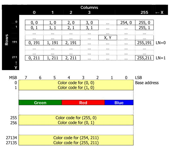
Pattern layout table base address is stored in register R#2, and corresponds to the cell (0, 0) in the picture above.
