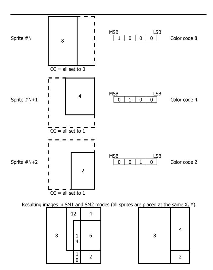
Sprite mode 2: CC flag is used, no collision detection
