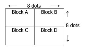
For each block A, B, C, and D sixteen colors can be specified. Two bytes are used for each pattern.
