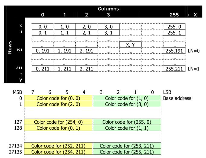
Pattern layout table base address is stored in register R#2, and corresponds to the cell (0, 0) in the picture above.
