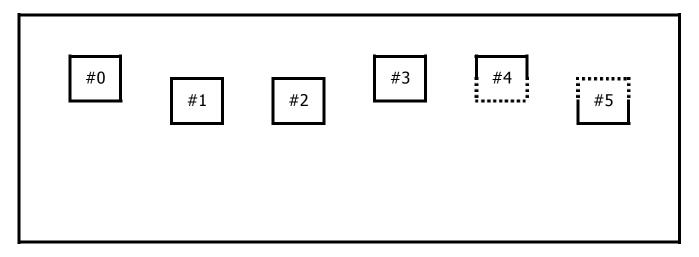
When two sprites collide (their pattern color 1 portions have overlapped), status register's S#0 bit 5 "C" is set to 1.
