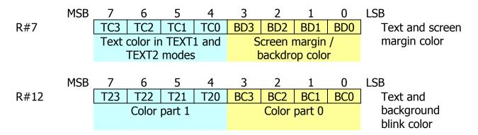
In TEXT2 mode, if attributes for blinking are set, color set in this register R#12 and in register R#7 are displayed alternatively (blinked).
