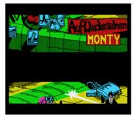
Offset screen\*, horizontal scan line is 256 dots, GRAPHIC1 mode, top appears at the bottom
