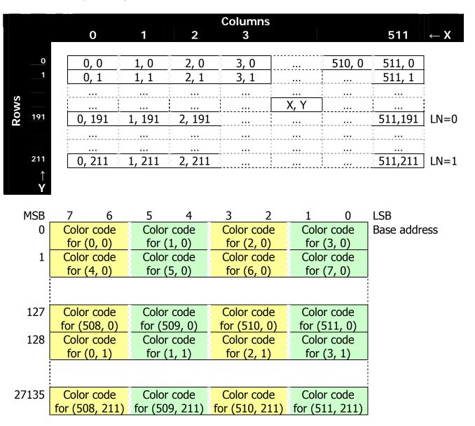
Pattern layout table base address is stored in register R#2, and corresponds to the cell (0, 0) in the picture above.
