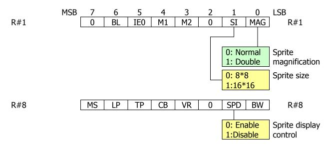
Sprites are defined by three tables: sprite pattern generator table, which controls the appearance of the dots within the sprite (being on "1" or off "0"), sprite color table, which control colors of the sprite lines and other attributes, and sprite attribute table, which controls positioning and used pattern number.
