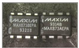
Figure 1. Valid Maxim part with correct grade B on the left and counterfeit part with grade A on the right. Note the evidence of the counterfeit rework on the vertical white line at the left side of the chip. There is a significant, diminished contrast between that white line and the new ink for the logo, date code, and part number. Note also the incorrect placement of the logo and date code.
