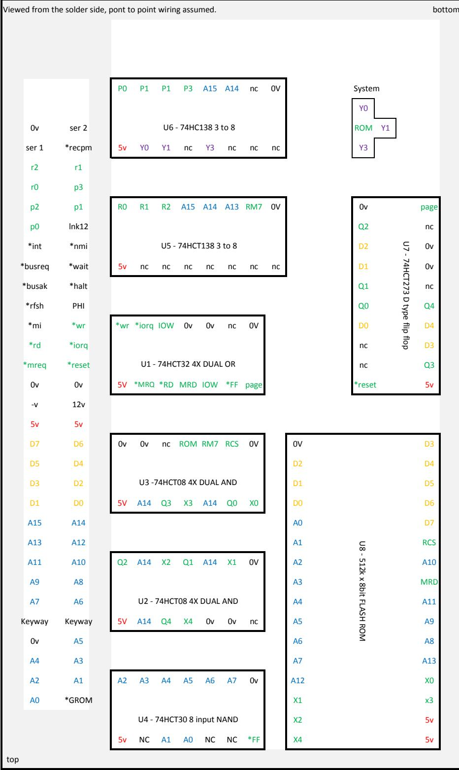
Version 3 tested & working, version 4 replaces the HCT20 with HCT30 to eliminate one of the HCT138's
