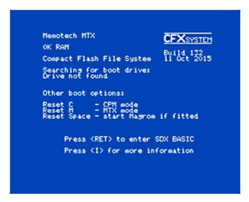
Holding down relevant key when the system is powered on or reset will enter the associated mode as shown. Pressing <**RET**> when the boot screen is displayed will enter SDX BASIC mode, or pressing <I> will display a crib sheet showing SDX BASIC USER disk commands
