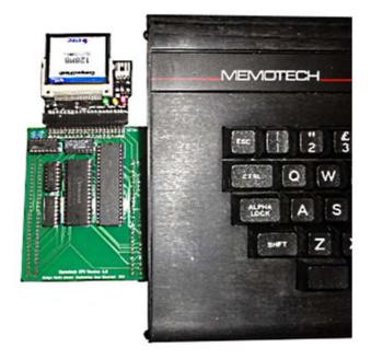
If you do not see the CFX Boot Screen, power off the system and check that the PCB has been correctly mated with the edge connector and that the CF Reader and Card are installed correctly.
