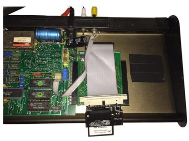
The CF Card Reader will sit on the base of the MTX, to ensure that there is no short circuits when the system is in use, insulate the base of the case - in this example, I have used insulation tape.
