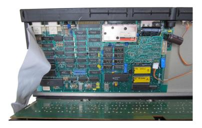
Gently ease the keyboard interconnecting cable from the mother board connector, always using the connector - do not pull on the ribbon cable.
