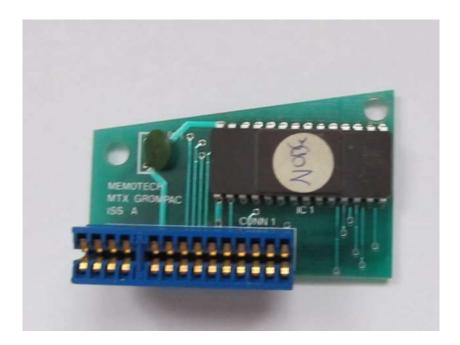
Anything other than a ROM board is likely to need multiple signals from the other half of the edge connector so in most cases it makes sense to fit the full 30 way connector. For mechanical stability if nothing else.
