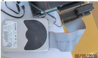
The wiring side, connections to the 82C55 I/O ports are in white, the data bus is yellow, address bus in blue and other control signals in green. Since the flash chip has 17 address lines, and only 14 are used, other are tied low. Which shows up in the photograph as apparently empty pins on the right side of the socket. Other than power very few wires needed to connect to more than 2 points.
