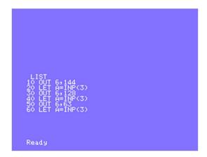
Lines 10 and 20 set the volume for tone 1 to maximum (144 is #90 hex or 1 001 0000 binary) Lines 30 and 40 set the low counter bits for tone 1 to zero (#80 hex or 1 000 0000 binary) Lines 50 and 60 set the upper counter bits to 63 so the count is 1008 and the output frequency 124hz or so. (#3F or 00 111111 binary).
