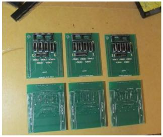
Using Port #FF could interfere with some of the other MTX hardware addons, most notably the Speculator. So, the board was modified to use the final NAND gate as another inverter so as to use port #FB instead, and it was this modified Version 5.1 that went on to become the V1.0 production board, seen here being assembled.
