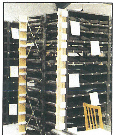
A 24-hour burn-in is standard along the assembly process. When the computer comes out of the box, it will work.
