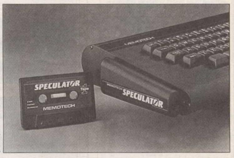
held in the memory, but has to be presented in a very different form to make sense to the MTX's video chip. The Rom pack sends interrupts to stop the game running, reads the Spectrum screen, translates it into values that produce the same on the Memotech screen, and sends the new data to the video chip. Fortunately pixel resolution is the same so the graphic details are reproduced exactly.
