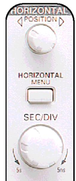
Figure 4: Horizontal Controls.
