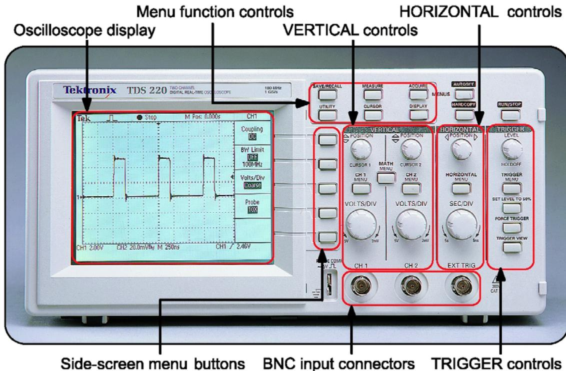
Figure 1: Front panel of a Tektronix TDS 220 oscilloscope.
