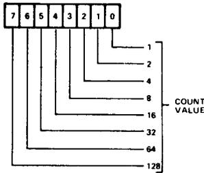
**WRITE** – 8 BITS LOADED INTO T1 LOW ORDER LATCHES. THIS OPERATION IS NO DIFFERENT THAT A WRITE INTO REG 4.
