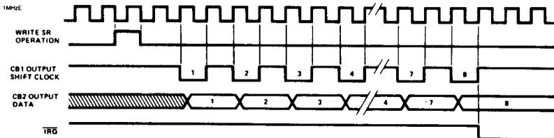
Figure 22.17 – Output Mode 6 Timing
