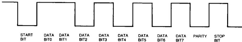
Fig 20.1 – Timing diagram for a serial character
