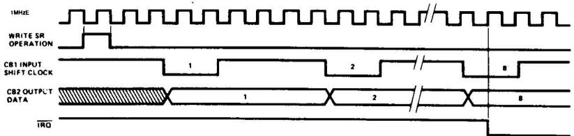
Figure 22.18 – Output Mode 7 Timing
