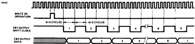
Figure 22.15 – Output Mode 4 Timing
