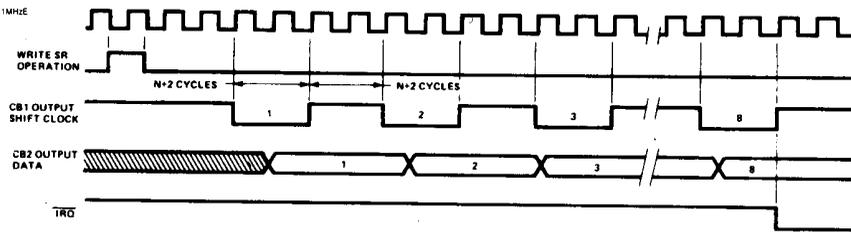
Figure 22.16 – Output Mode 5 Timing
