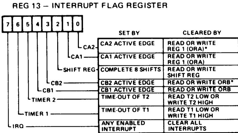
\* IF THE CA2/CB2 CONTROL IN THE PCR IS SELECTED AS "INDEPENDENT" INTERRUPT INPUT, THEN READING OR WRITING THE OUTPUT REGISTER ORA/ORB WILL NOT CLEAR THE FLAG BIT. INSTEAD, THE BIT MUST BE CLEARED BY WRITING INTO THE IFR, AS DESCRIBED PREVIOUSLY.
