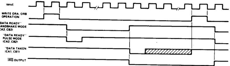
Figure 22.5 – Write Handshake Timing
