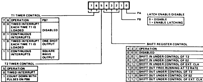
Figure 22.10 – Auxiliary Control Register
