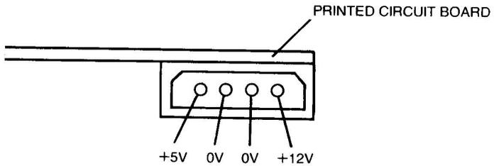
Figure H.2 – Typical disc drive power connector
